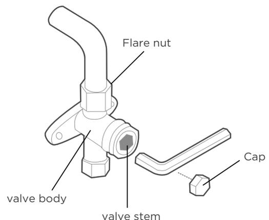
12. Using hexagonal wrench, fully open both the high pressure and low pressure valves.
