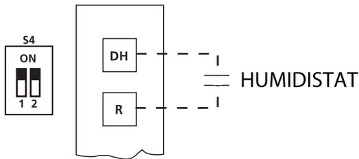
Dehumidification control requires external Humidistat at DH and R. Set S4-2 as OFF. When the humidity rises and exceeds the set value of the Humidistat, the 24V signal of DH changes to 0V, the cooling system starts the dehumidification operation, and the air volume drops to 80% of the nominal cooling air volume.
