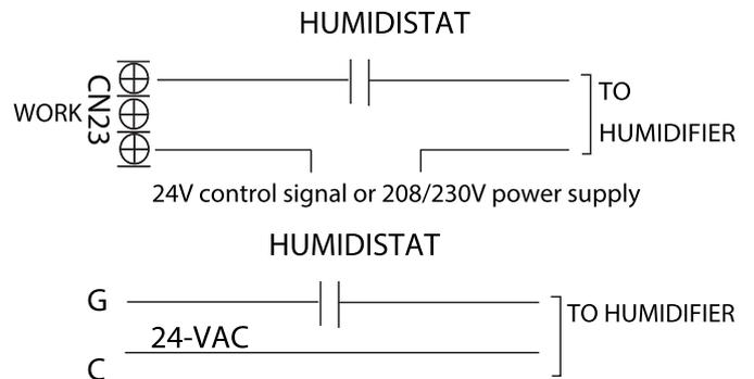
To connect a humidifier, utilize the passive signal "WORK" output (CN23) port as well as the G and C wires on the controller, and wire the humidistat and humidifier per above wiring diagram. When the fan is running, the CN23 relay will be closed, which will allow power to the humidifier when the humidistat is below humidity setpoint. If the thermostat or zone controller has an HUM interface, connect the humidifier directly to the HUM and C ports.
