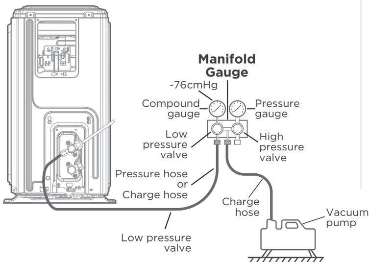
6. Close the Low Pressure side of the manifold gauge, and turn off the vacuum pump.
