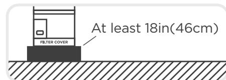
☑ Place air handler so that heating elements are at least 18 inches (46 cm) above the floor for a garage installation. Failure to follow these instructions can result in death, explosion, or fire.
