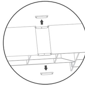
Remove knockouts as shown in the figure.
