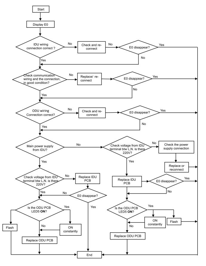
**Remark**: if the communication wiring **1(S)** is not well connected, the ODU LED5 will light **ON** always.
