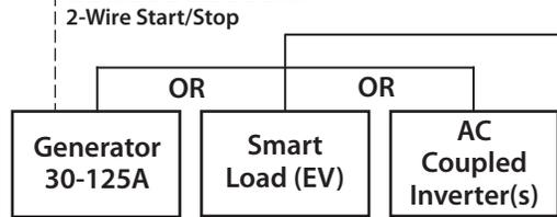
Distribution Breakers for the dedicated Gen Port Combiner Panel should be sized to distribute total Input amperage evenly up to 50 Amp per inverter. For example if you have a 60 Amp rated Generator then the main breaker would be 80 A and each inverter breaker would be 30 Amps for 3 inverters (20A x 1.25 & next size).
