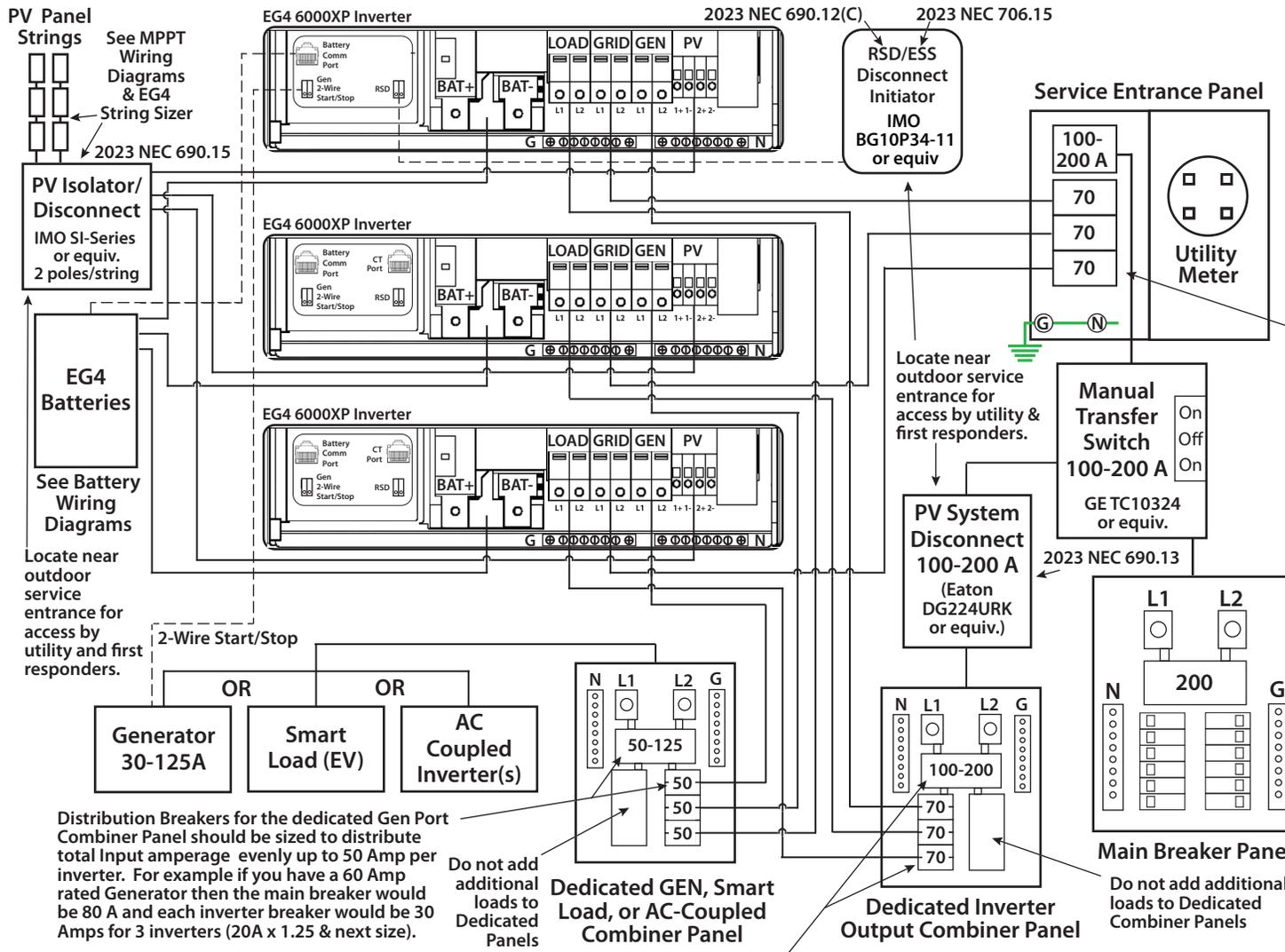
**IMPORTANT NOTE:** The EG4 6000xp inverter is not capable of providing sell-back power to the utility. It is only a backup or off-grid inverter with the capability of grid INPUT for charging batteries or passing through grid power through the load port to a critical loads subpanel or transfer switch. It is essentially a battery charger. Therefore it is not regulated by the NEC 705 (2023) Interconnection code.
