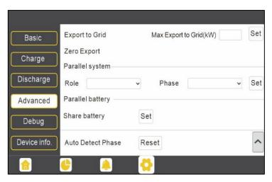
"Role" setting of the parallel system. It is set to "1 phase master" by default. In a parallel system, only one inverter is allowed to be set as Master and the others are set as Slaves.
