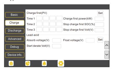
**Charge first power (kW):** Limits PV charge *power*
