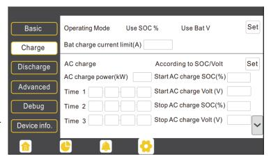
**Charge first (PV):** PV charge configuration. When using 'Charge first,' PV will charge the battery as the priority. Users can set up to three different time periods when PV charge can happen.
