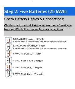
Two positive 1/0 and two negative 1/0 battery cables (minimum 215 amps) from busbars to inverter terminals are required otherwise battery breakers will trip at higher loads.
