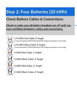
Two positive 1/0 and two negative 1/0 battery cables (minimum 215 amps) from busbars to inverter terminals are required otherwise battery breakers will trip at higher loads.
