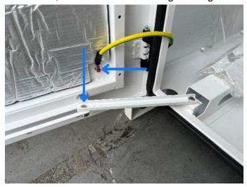
Using pliers, release the three sets of pins (top and bottom on each hinge) securing the door to the cabinet.
