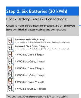
(minimum 215 amps) from busbars to inverter terminals are required otherwise battery breakers will trip at higher loads.
